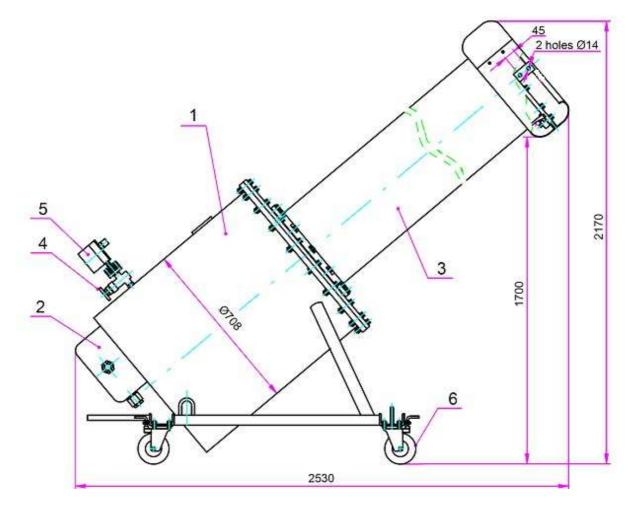
1 - tank; 2 - cover; 3 – glass-epoxy cylinder; 4 – bellows valve; 5 – pressure gauge; 6 – roll.
